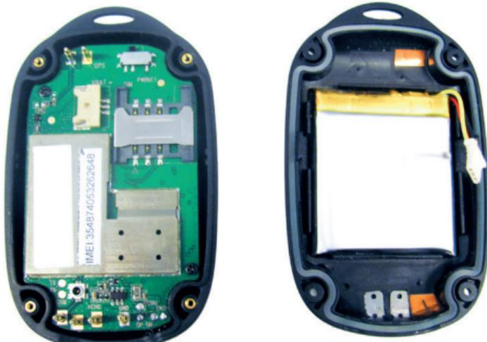
The product comes in an unlocked state, allowing you to install the required SIM card without having to unscrew anything. Please make sure the SIM card is not locked by a PIN code.
