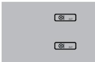
during a call, press the
