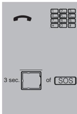
leave the receiver on the telephone and use the keypad to enter the phone number (up to 20 digits)
