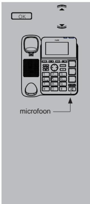
press the **OK** button again and use the **▲** and **▼** buttons to select **RECORD** press the **OK** button and record your notification text after the beep tone
