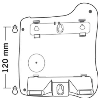
2. Hang the telephone with the key holes on the screws and push the telephone downward.
