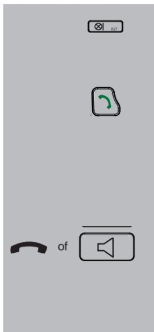
during a call with the outside line, press the **INT**(\*) button; the wireless handset will start ringing
